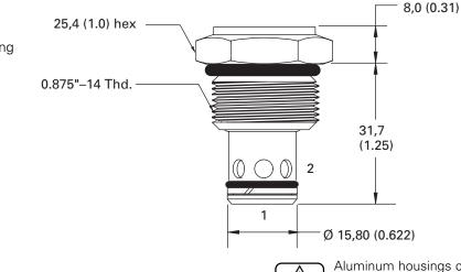
Aluminum housings can be used for pressures up to 210 bar (3000 psi) Steel housings must be used for operating pressures above 210 bar (3000 psi)
