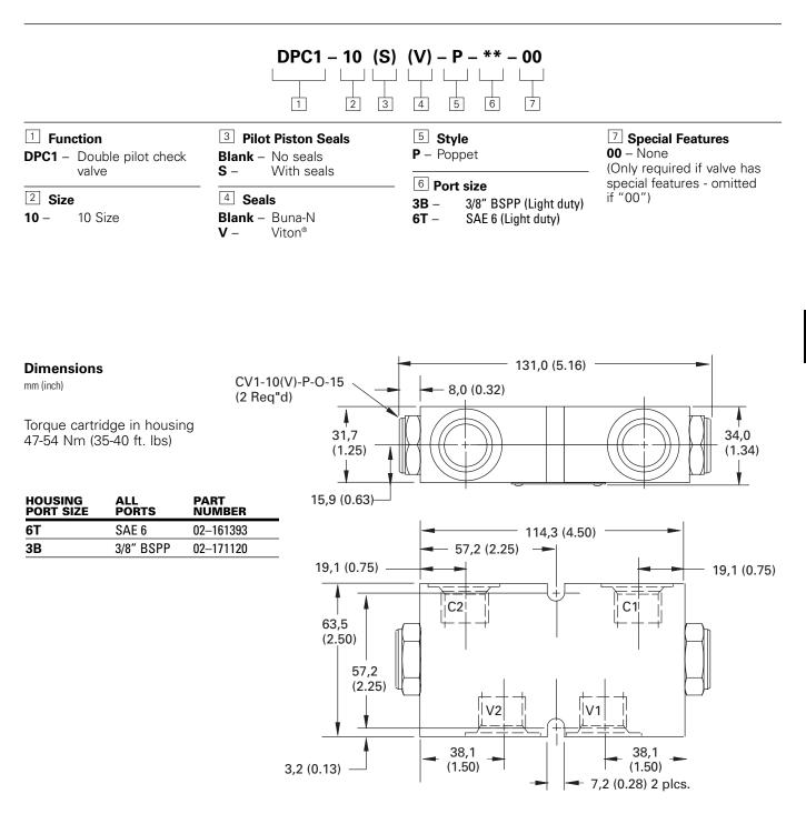
The DPC11-12 is an inline housing type, double pilot operated check valve.
