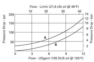
A – Port V to C (free flow) **B** – Port C to V (pilot open)
