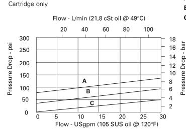
**A** – CV11-12-P-O-80 **B** – CV11-12-P-O-20 **C** – CV11-12-P-O-2.5
