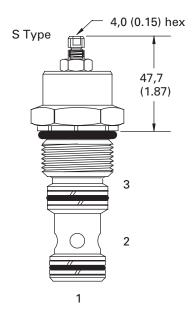
The DPC2-8 is a Pilot-to-Open, screw-in cartridge type, dual pilot operated check valve.
