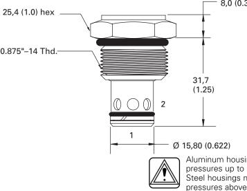
Aluminum housings can be used for pressures up to 210 bar (3000 psi) Steel housings must be used for operating pressures above 210 bar (3000 psi)
