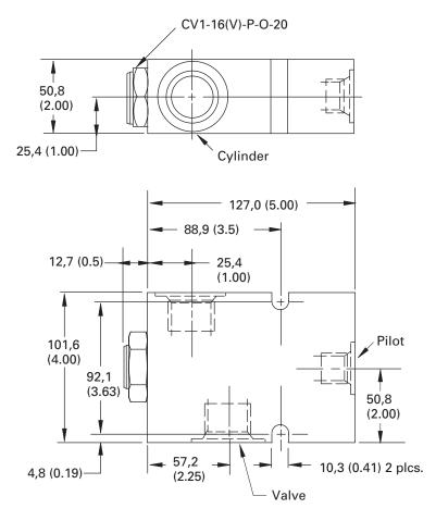
The SPC1-20 is an inline housing type, pilot-to-open check valve.
