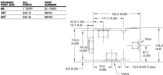
The POC1-10 is a pilot-toopen, screw-in cartridge type check valve.
