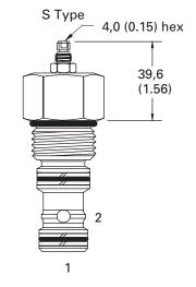
The POC1-12 is a pilot-toopen, screw-in cartridge type check valve.
